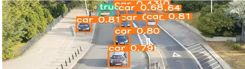
Figure 5. Vehicle detection using YOLOv8
