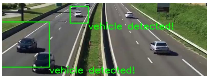
Figure 4. Vehicle detection using Haar Cascade classifier
