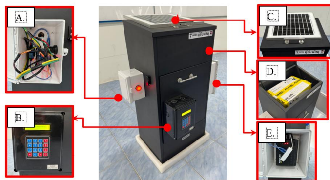
Figure 2. Five parts used for system: part A: detecting parcel; part B: keypad door lock; part C: solar cell; part D: serves as the parcel drop-off section; and part E: battery of system
