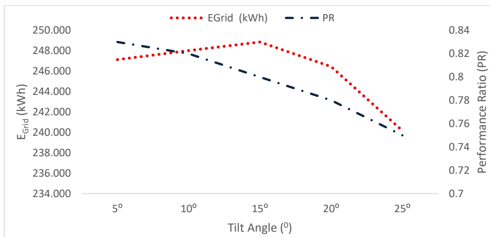
Figure 7. Comparative visualization of the relationship between tilt angle, E_{Grid} , and PR
