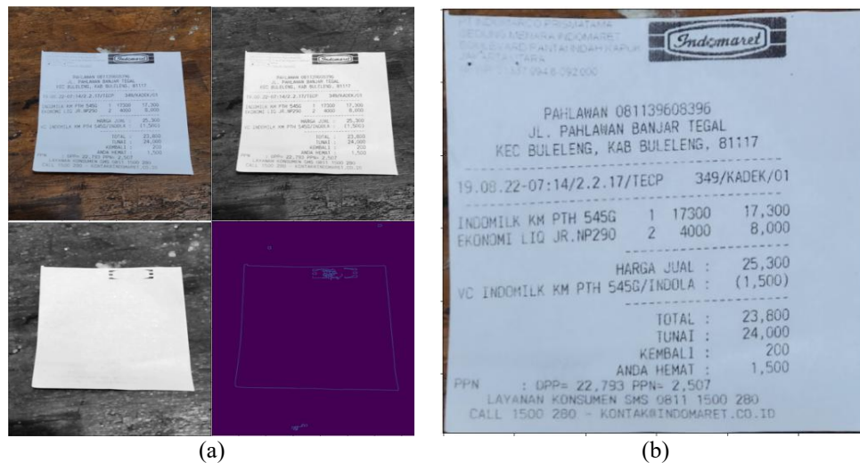
Figure 2. The ROI segmentation process; (a) data processing: original (top left), grayscale (top right), blur and dilated (bottom left), contour edge (bottom right) and (b) ROI cropping result
