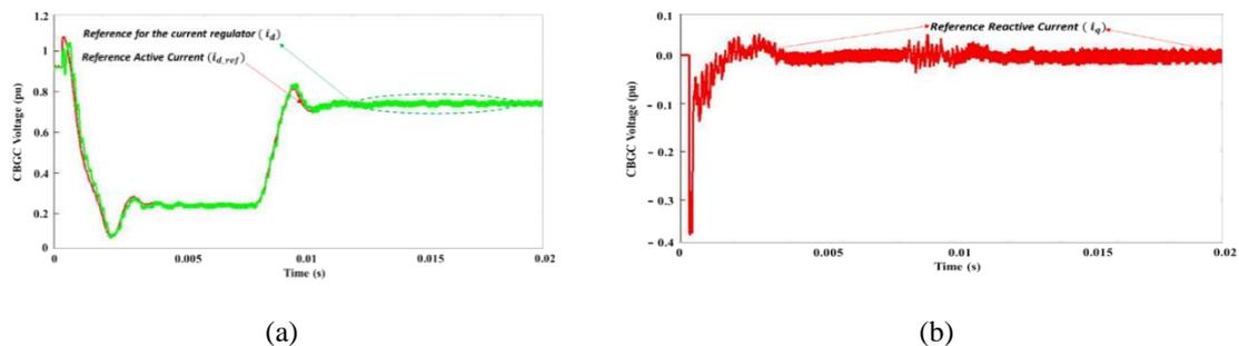
Figure 22. The controller of the CBGSC reference, (a) active, (b) reactive currents
