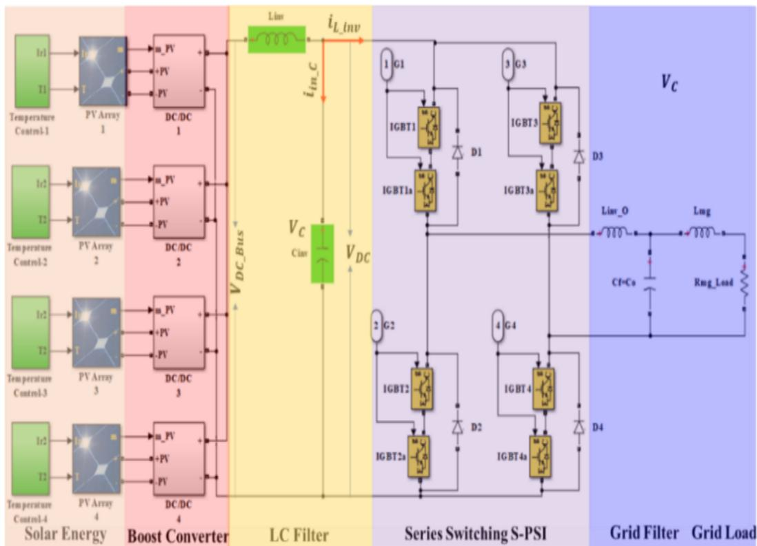
Figure 1. Proposed series switching SPSI circuit configuration [1]
