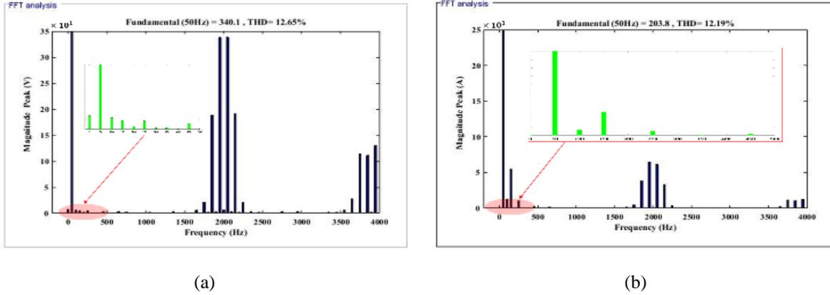
Figure 17. FFT analysis of the S-PSI, (a) voltage, (b) current THD waveforms without filtering [1]
