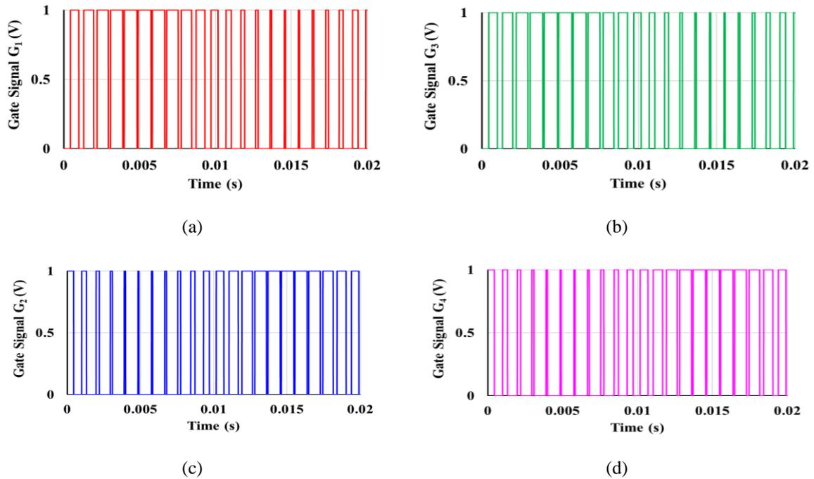
Figure 10. Separate comparator circuits signals ( $G_1, G_3, G_2$  and  $G_4$ ) for SPSI
