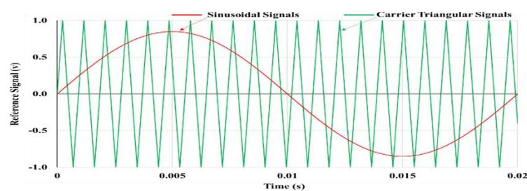
Figure 9. Reference sinusoidal and carrier triangular signal waveforms
