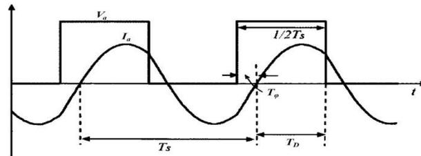
Figure 8. Half phase PSI voltage and current [22]
