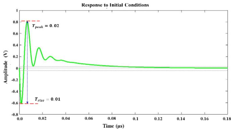
Figure 11. The step response waveform of the IGBT switch to the initial condition
