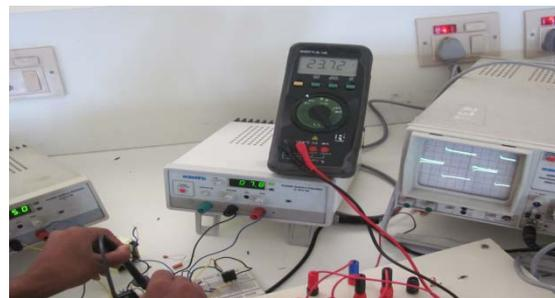
Figure 8. Experimental Set-up for the High Gain IBC
