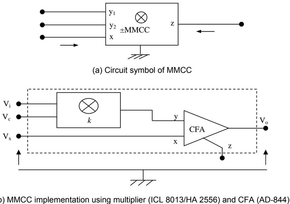
Figure 1. The Multiplication Mode Current Conveyor (MMCC)
