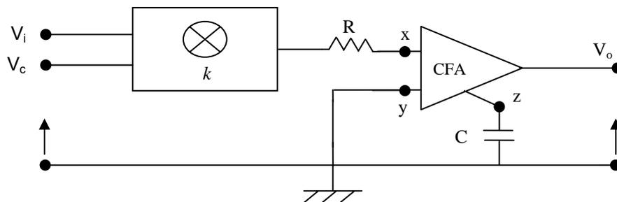
(b) Alternate inverting integrator with  $+V_c$
