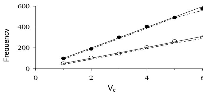
(c) Linear tuning characteristics with  $C=150$ pF:  $R = 1K\Omega$  (●) ;  $R=2K\Omega$  (○) (dotted line by hardware test)
