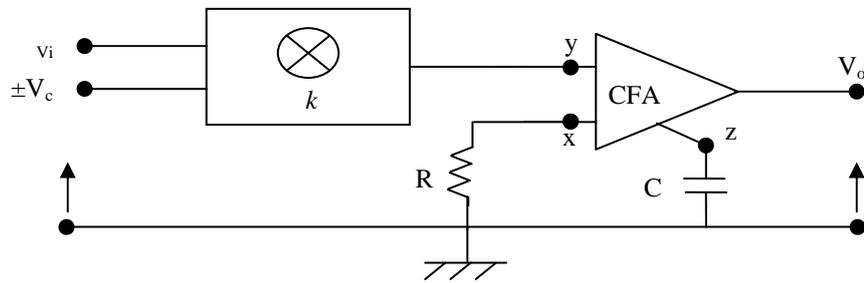
(a) Either polarity integrator design with  $\pm V_c$
