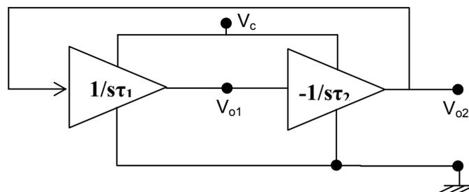
(c) Double integrator loop sinusoid quadrature-signal output ( $V_{o1}$  &  $V_{o2}$ ) oscillator
