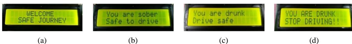
Figure 5. LCD display during, (a) System start up, (b) Sober, (c) Mildly drunk, and (d) Drunk
