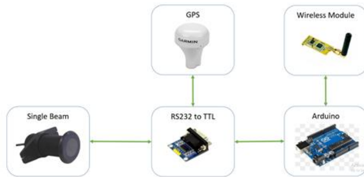
Figure 2. The architecture of the ASV communication system
