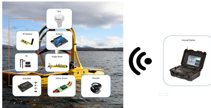
Figure 1. Overall system design of ASV for SAR
