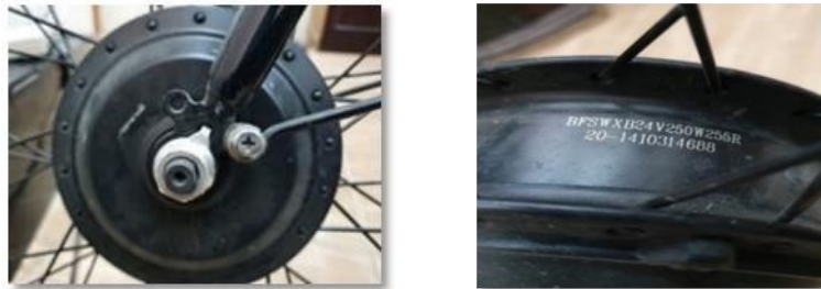
Figure 3. DC motor of e-bike
