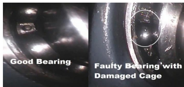
Figure 3. The good and defective bearing used for analysis for wireless CM
