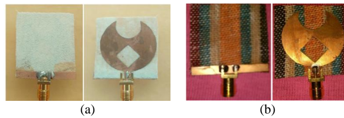
Figure 2. The antenna (a) flannel fabric and (b) jeans fabric [42]
