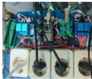
Figure 8. Control system in smart hydroponics
