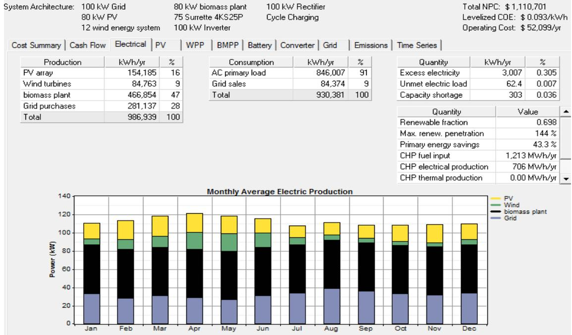
Figure 10. Contribution of electrical energy production by PV/wind/biomass/grid substation
