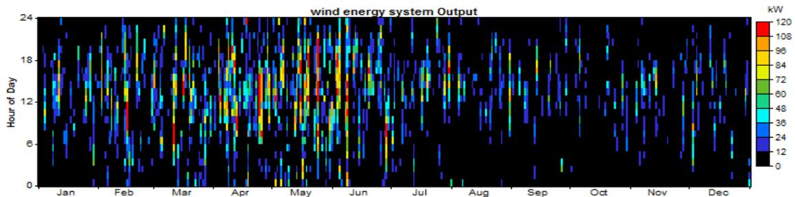
Figure 12. Annual electric energy production by wind energy system
