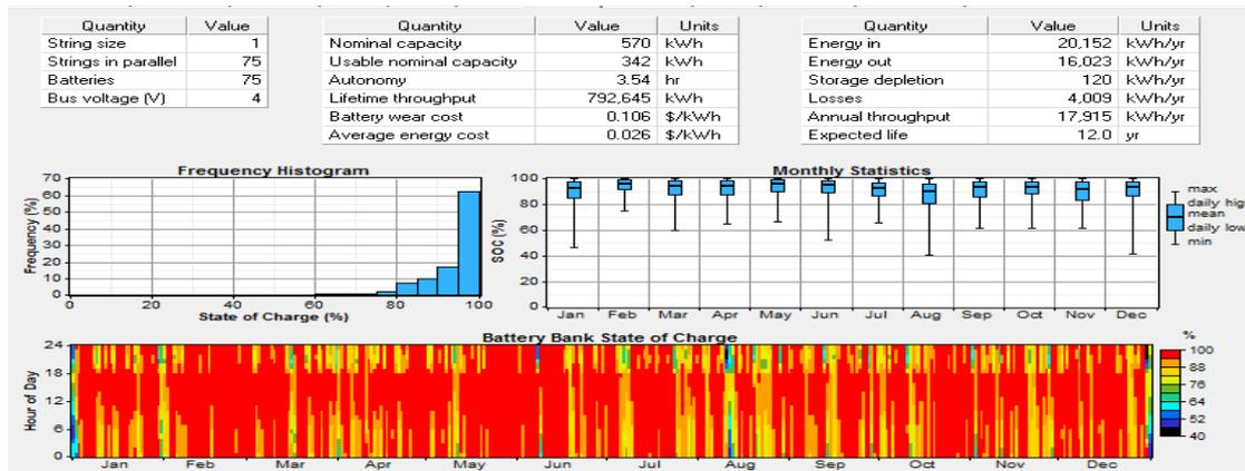
Figure 14. Statistical result of battery system
