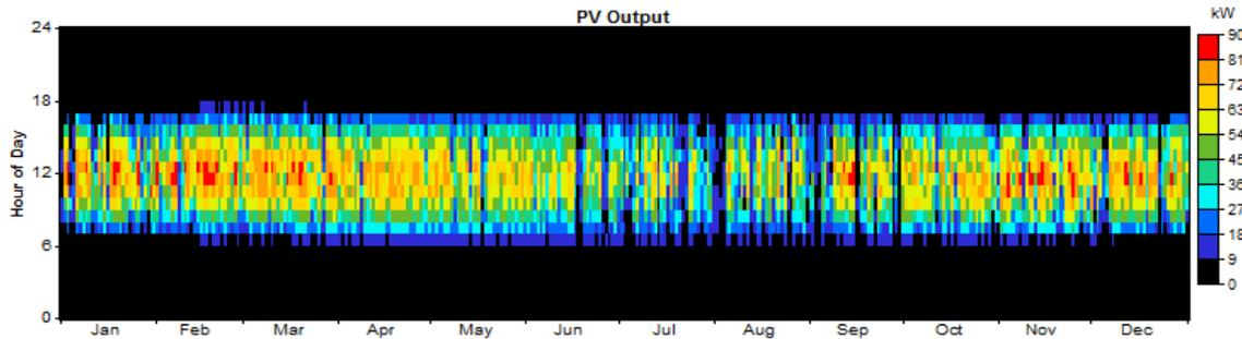
Figure 11. Annual electric energy production by PV system
