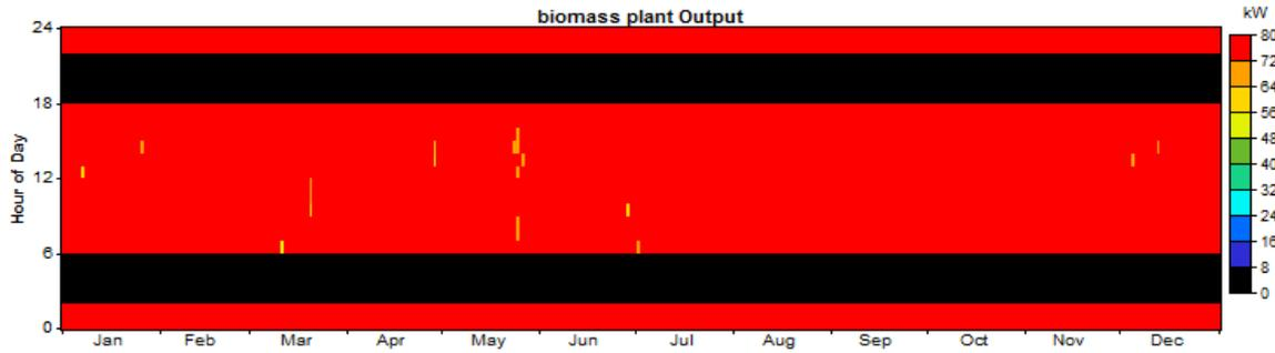
Figure 13. Annual electric production by biomass energy system
